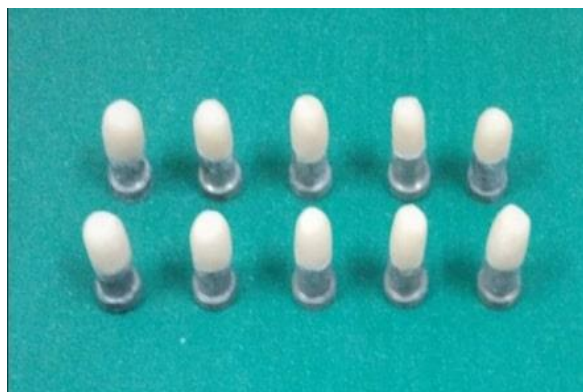
Fig 2. Samples for Shear bond strength test
