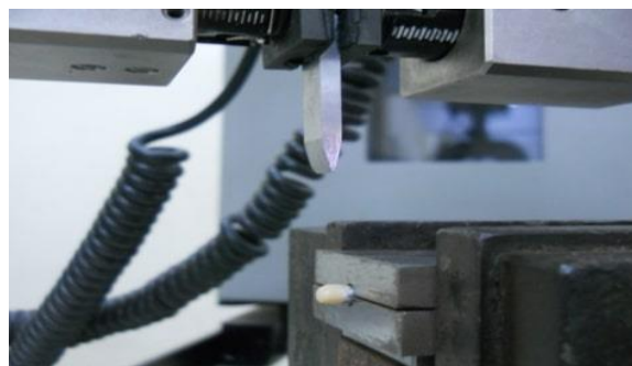
Fig 4. Shear bond strength test
