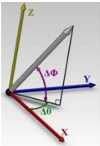
Fig. 3: Horizontal ( $\Delta\theta$ ) and vertical ( $\Delta\Phi$ ) angles
