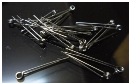
Fig. 1. A 1.5 mm diameter stainless steel ring made of 0.5 mm orthodontic wire with two additional arms for better handling.
