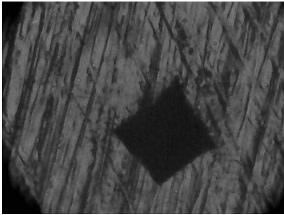
Fig. 1. Indentation made with the Vickers hardness machine
