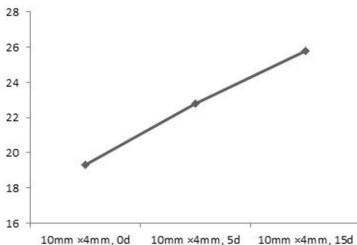
**Fig. 4.** Gradual increase of stress on implant (10mm×4mm) by increase of angle.
