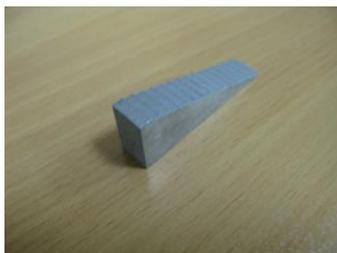
Fig. 1: Aluminum step wedge
