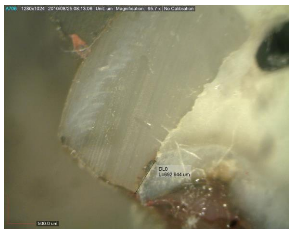
Fig. 1: Measurement of dye penetration depth into a tooth section under a stereomicroscope at \times 10 magnification
