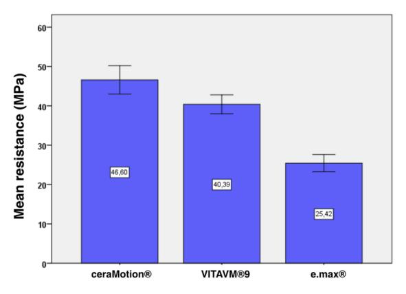
**Fig. 1:** Representation of the mean fracture toughness (MPa) of ceraMotion® Zr, VITA VM®9, and IPS e.max® veneering ceramics (n=number of samples; the error bars represent 95% confidence interval (CI) of the mean)
