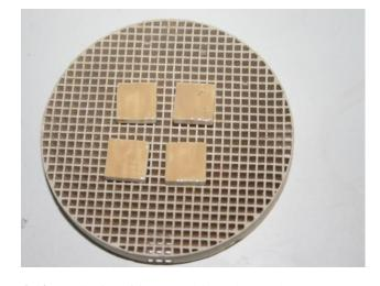
Fig. 2: Application of liner porcelain on the samples
