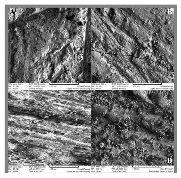
**Fig. 6:** SEM topography microphotographs ( $\times$ 500 magnification), (A) Al<sub>2</sub>O<sub>3</sub> air abrasion, (B) CO<sub>2</sub> laser irradiation, (C) Er:YAG laser irradiation, (D) Control group. Note the cracks in the melted surface (decreased micro-roughness) of the laser-irradiated groups and the abrasion lines in the air-abraded group
