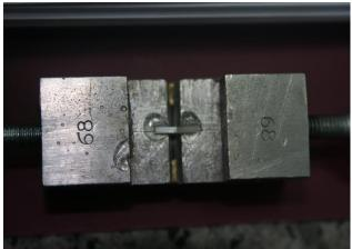
Fig. 3: (A) Microtensile bond strength tester machine. (B) The sample in the microtensile bond strength tester machine
