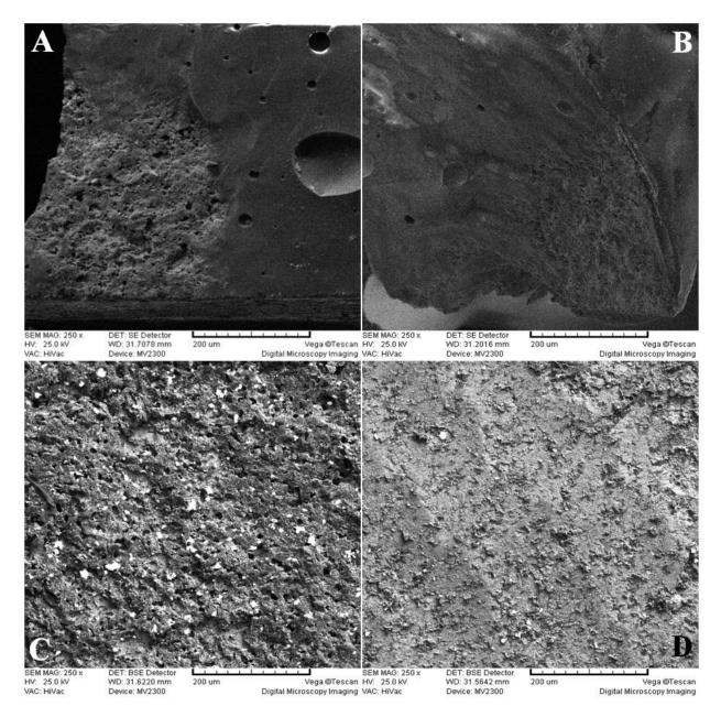
Fig. 5: SEM microphotographs of the fractured surfaces: (A)  $Al_2O_3$  air abrasion, (B)  $CO_2$  laser irradiation, (C) Er:YAG laser irradiation, (D) Control group. Note the mixed fracture patterns in all the study groups
