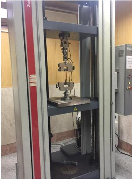
**Fig. 2:** Universal testing machine
