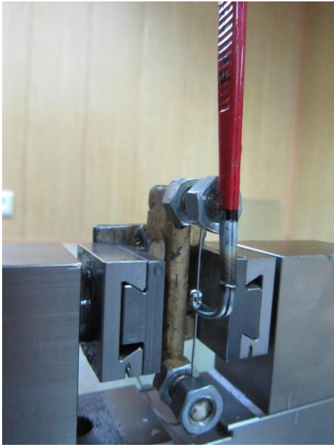
Fig. 1: The cling-shaped device used for holding the bracket during the upward movement of the superior jig of the testing machine
