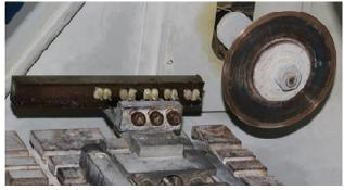
Fig. 2: Sectioning of the mounted samples
