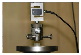
Fig. 3: Push-out test
