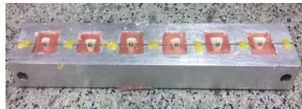
Fig. 2. Acrylic blocks containing teeth prepared for shear bond strength testing
