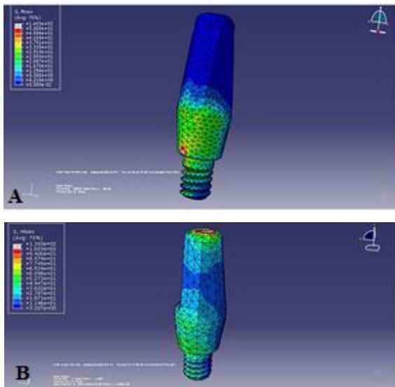
**Fig. 4.** (a) Stress distribution pattern in abutment during static loading; (b) stress distribution pattern in abutment during cyclic loading; (c) stress pattern in abutment during 60 s of masticatory cycles
