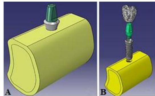
**Fig. 1.** (A) Implant-abutment assembly; (B) load and boundary conditions of the 3D finite element analysis model
