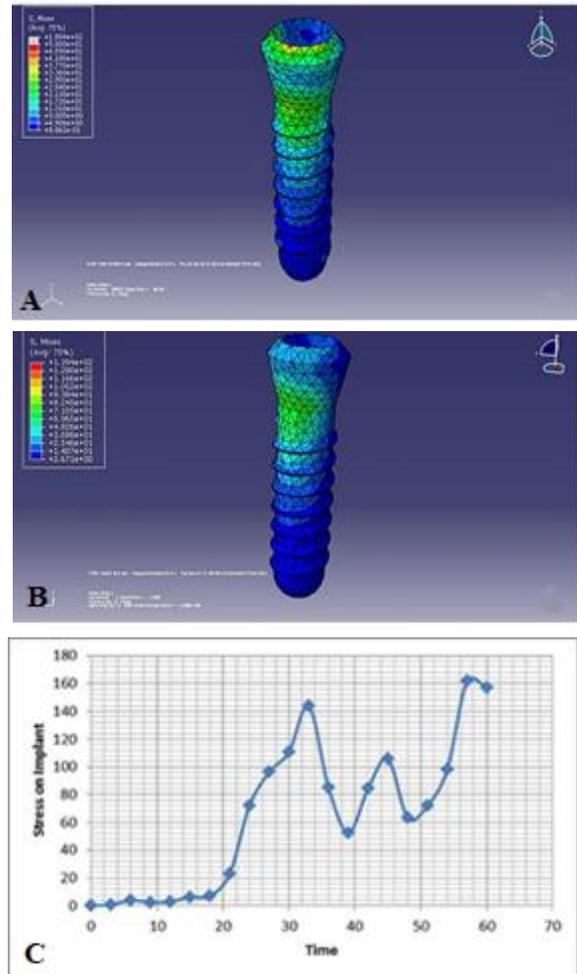
**Fig. 3.** (A) Stress distribution pattern in implant during cyclic loading; (B) stress distribution pattern in implant during dynamic loading; (C) stress pattern in implant during 60 s of masticatory cycle
