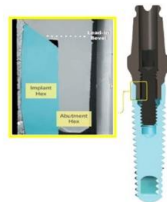
Fig. 2. Slip joint connection in Zimmer implant
