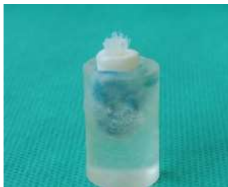
Fig. 4. Group 3 custom-made braided glass fiber posts
