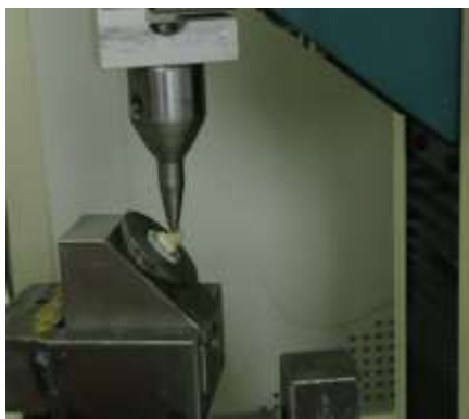
Fig. 5. Application of force at 135° angle relative to the tooth longitudinal axis in a universal testing machine
