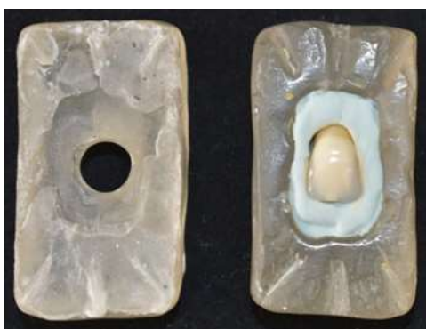
Fig. 1: Transparent acrylic resin mold with a tooth positioned in the central part in silicone material
