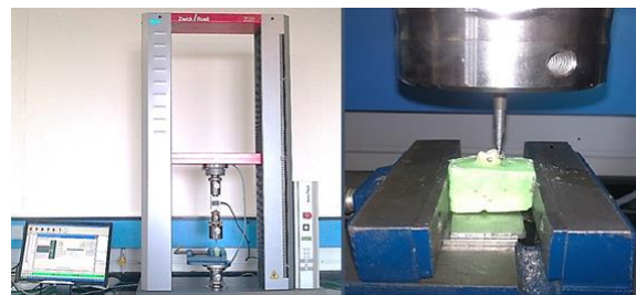
Fig. 2: Performing the shear bond strength test using a universal testing machine
