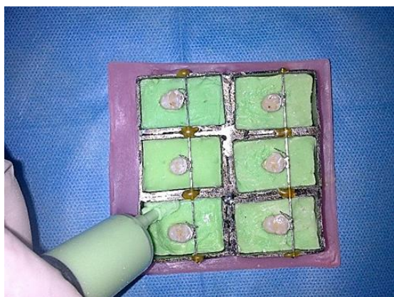
Fig. 1: Fixing the teeth in a metal mold in an appropriate direction using a 0.016×0.022-inch wire
