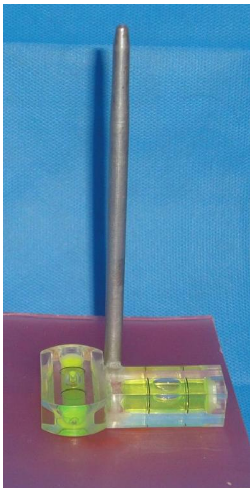
Fig 1. THIP is a single pin that is attached perpendicular to the two bubble style levels while they are in true horizontal position (bubbles placed in central position).
