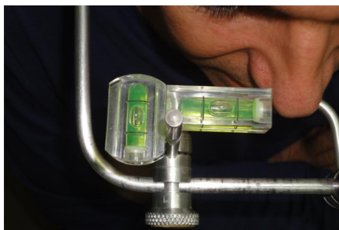
Fig.. 2- 3. THIP is adjusted to the true horizontal plane (bubble style levels placed in central position).
