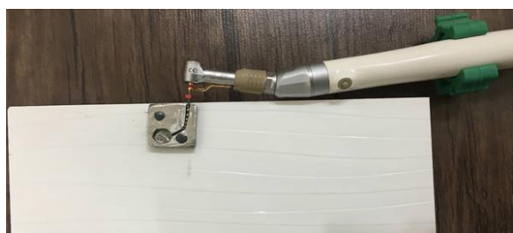
Fig. 1: Designed device to measure the cyclic fatigue resistance of the files
