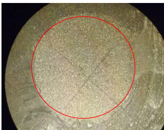
Fig 1. Depicts the adhesive failure between the cement and alloy.
