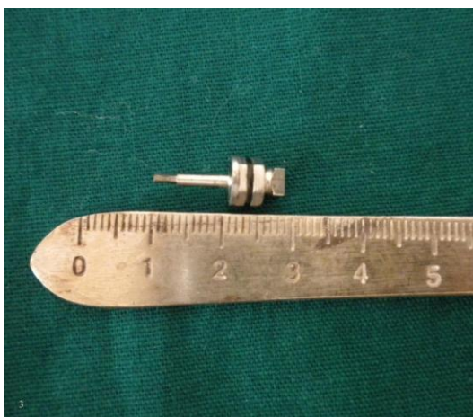
Fig 3. Retrieved 19 mm long implant screw driver.
