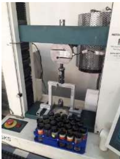
Fig. 1. Custom-made device for placement of bracket and wire sets in the universal testing machine
