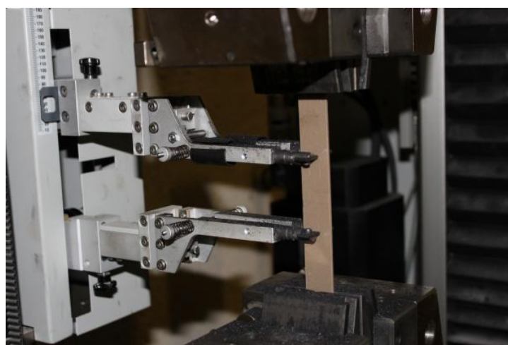
Fig 6. The universal tensile strength measurement machine with a rectangular specimen
