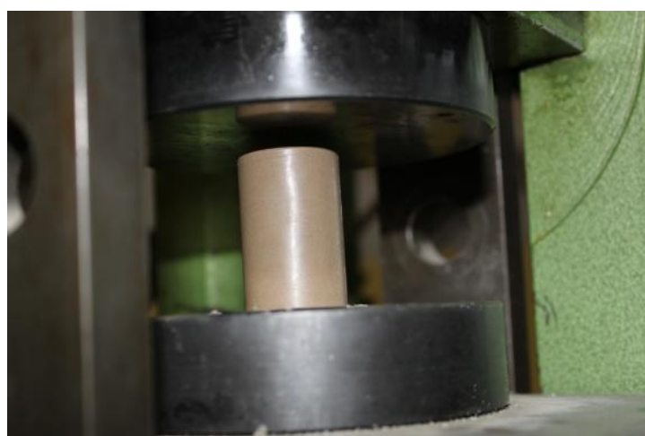
Fig 5. The compressive strength measurement apparatus with a cylindrical specimen
