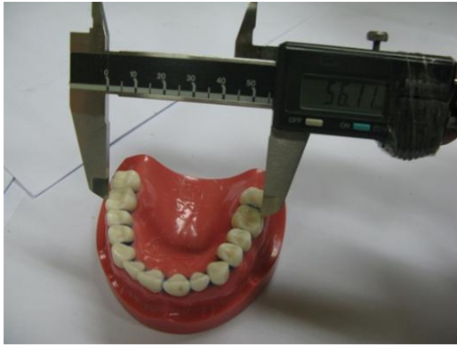
Fig 1. Cross-arch width (facial surface of the right first molar to the facial surface of the left first molar)
