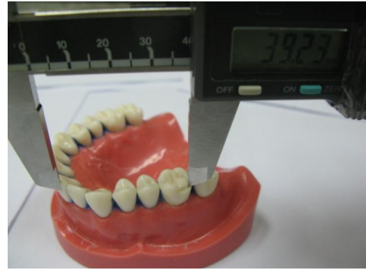
Fig 2. Antero-posterior measurement (distal surface of the right first molar to the labial surface of the central incisor on the same side)
