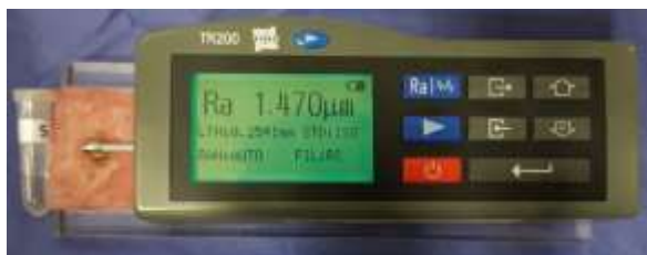
Fig. 1. Determination of surface roughness of samples (Profilometri System)
