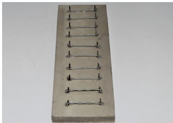
Fig 1. Handmade jig made from two rows of steel pins with a 25mm distance.
