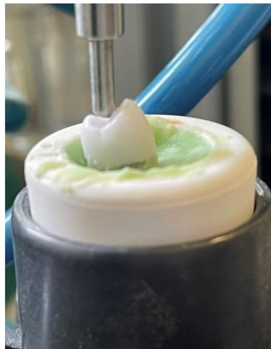
**Fig. 1.** Load application to a crown in a universal testing machine
