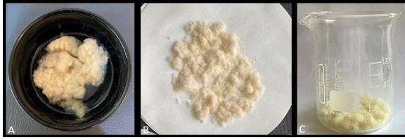
Fig 1. Natural wool fibers: (A) After cutting and before ultrasonic cleaning, (B) after ultrasonic cleaning and drying for 24 hours on filter paper, and (C) after silane treatment and drying for 14 days.
