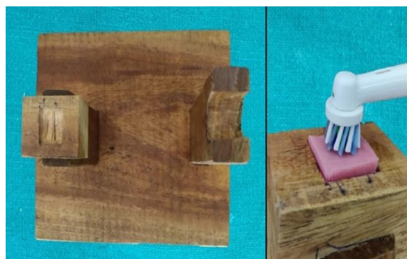
Fig 2. A customized wooden jig to standardize the brushing protocol: A wooden jig with two vertical pillars with a customized toothbrush-holding depression (for the selected toothbrush – Oral B Pro 2000N) and a specimen-holding platform was designed to standardize the brushing protocol.
