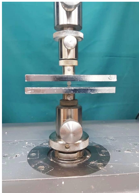
Fig 2. A specimen positioned in a universal testing machine for the assessment of diametral tensile strength.
