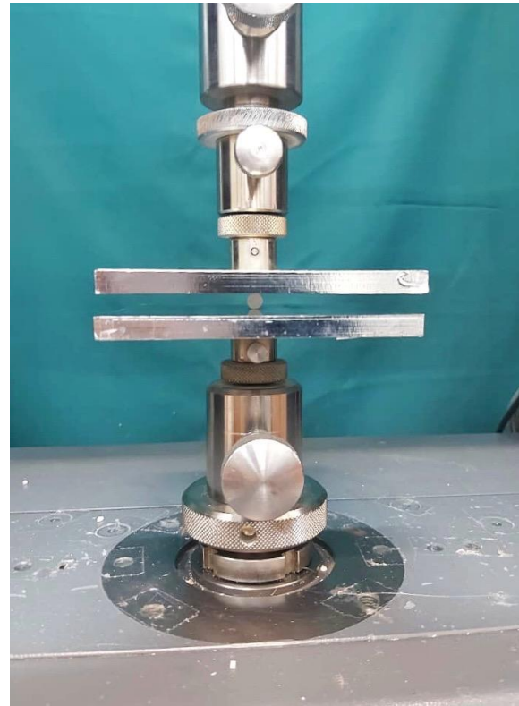
Fig 2. A specimen positioned in a universal testing machine for the assessment of diametral tensile strength.
