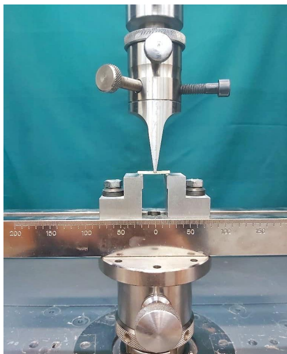
Fig 3. A specimen mounted in a universal testing machine for evaluation of flexural strength.
