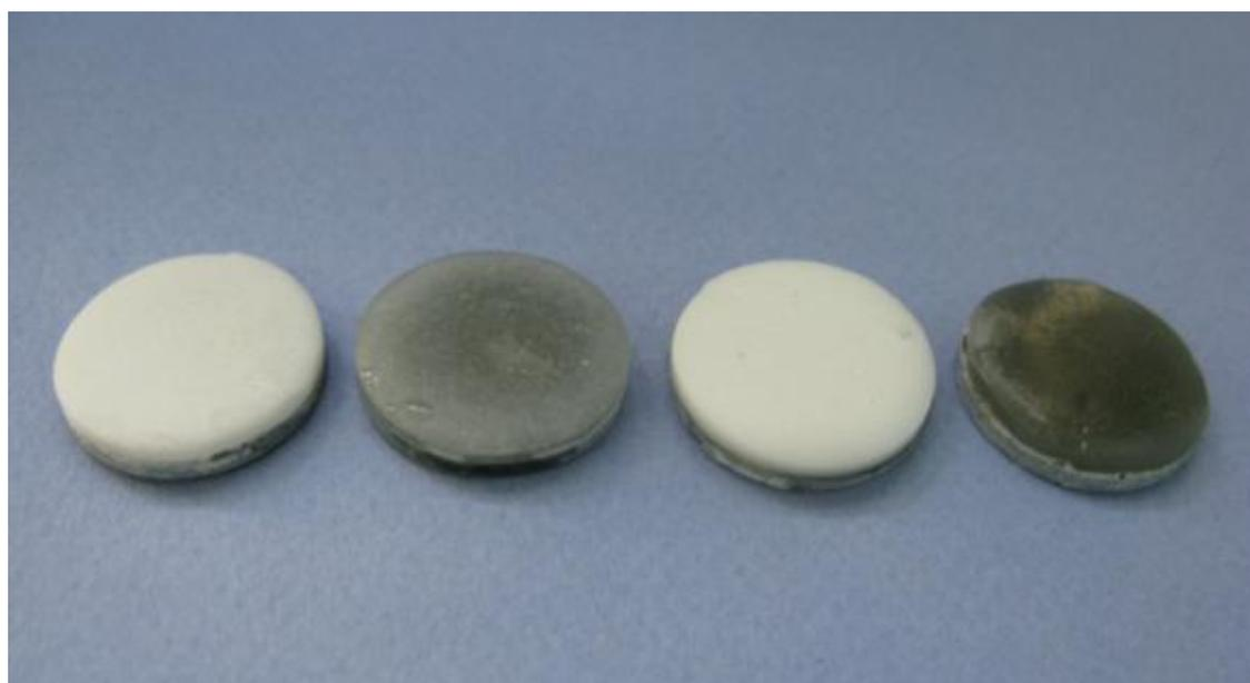
**Fig 4.** Specimen samples of four tissue-conditioning materials layered with modeling plastics
