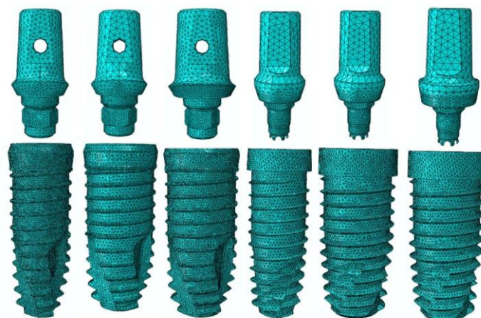
Fig 1. Three dimensional models of implants and abutments. From left to right: model XiVE a, model XiVE b, model XiVE c, model 3i a, model 3i b, and model 3i c.
