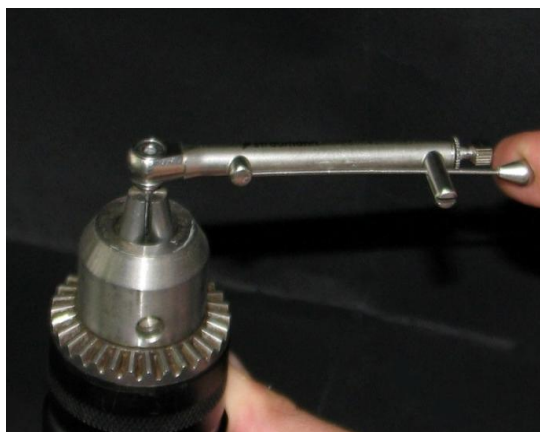
Fig 3. Practitioner exerting tightening abutment torque to the head of the screw driver
