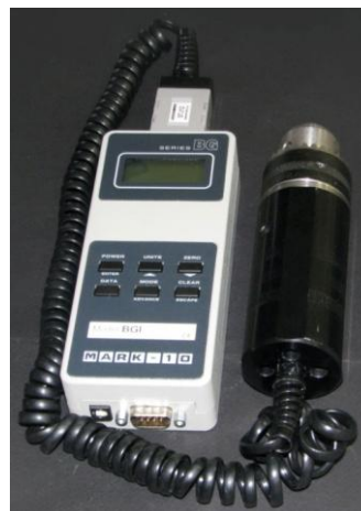
Fig 2. Mark-10 digital force/torque indicator model BGI
