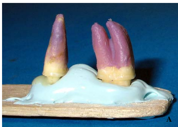
Fig. 2: Teeth were placed in the index (A), for embedding into acrylic resin (B)
