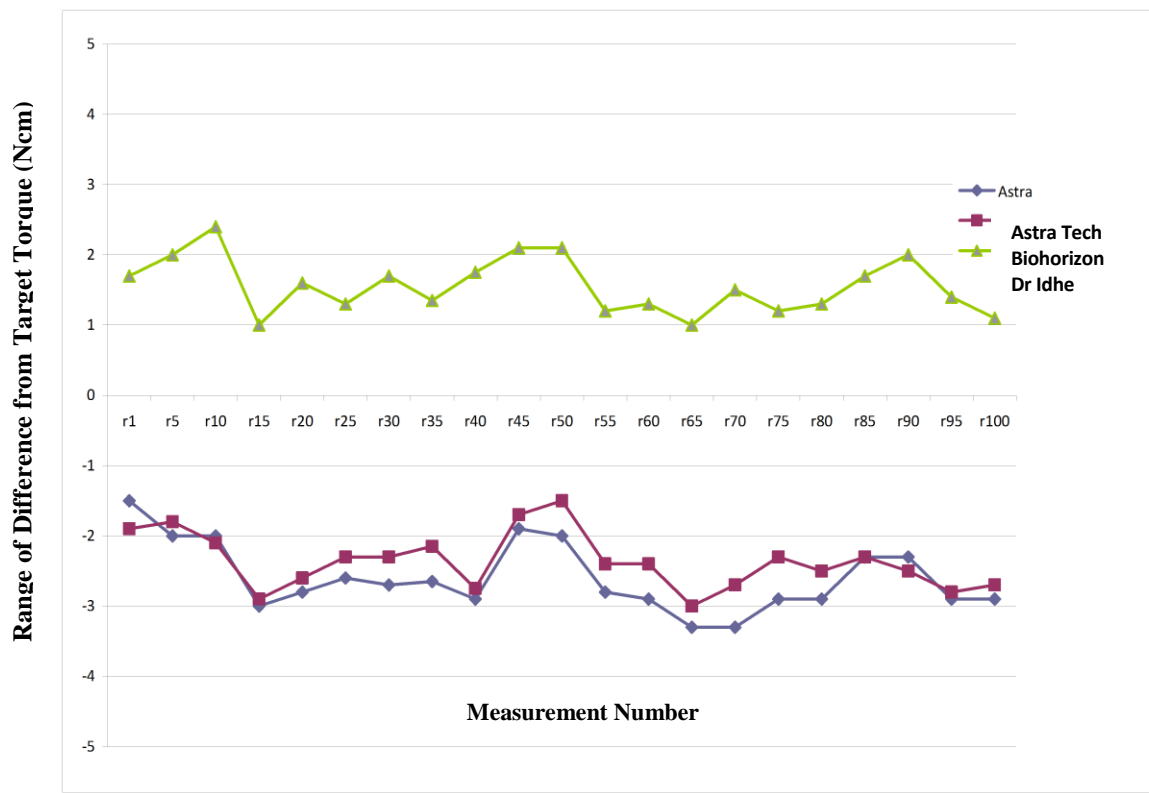
Fig4. Mean of difference between peak torque and target torque values, during one to hundred times of measurement for 3 groups of friction-style mechanical torque limiting devices tested after aging. Zero level, showing target torque for three Astra Tech, Biohorizon and Dr Idhe groups
