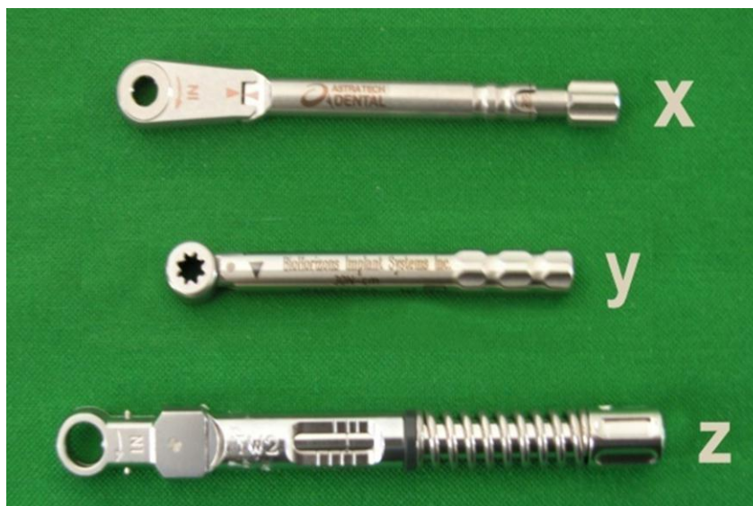
Fig 1. The friction-style mechanical torque limiting devices tested.
