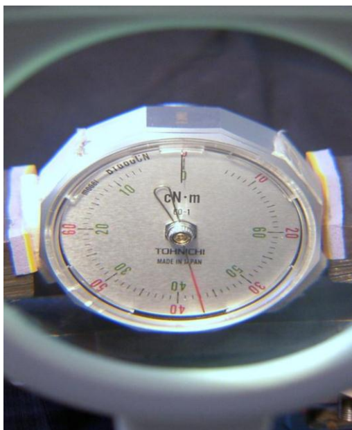
Fig 2. The peak torque values of each friction-style mechanical torque limiting devices (F-S MTLDs) presented on the torque indicator of the gauge for each device were registered using a magnifier
