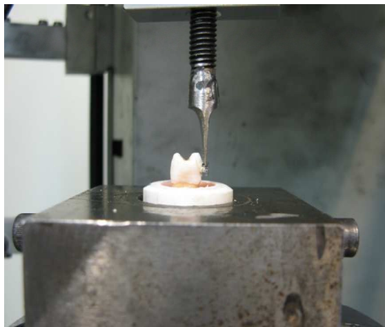
Fig1. Tooth mounted in the universal testing machine
