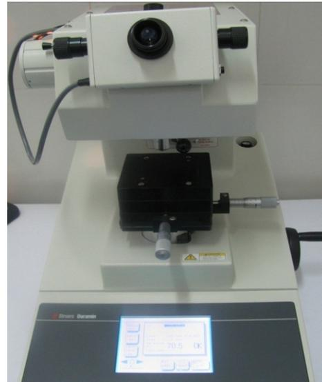
Fig 4. Vicker's microhardness device
