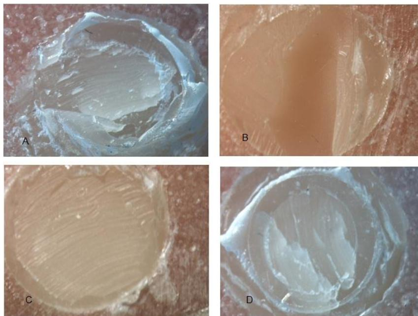
**Fig. 1.** Stereomicroscope images of Fracture patterns ( $\times 20$ ) which are classified as: A: cohesive in the repairing composite resin, B: cohesive in the repaired composite resin, C: adhesive, and D: mixed
